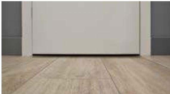
Doors with undercut dedicated to the MVHR system are available in models: CAMBIO, SIMPLE, TIARA, INTER-AMBER, IMPULS, SONATA, DECO, DECO LUX, HARMONY, SUBLIME, ANMI, VILANO, VERTIGO, FIORD, MODERN, MODENA, HAPTIC. The door leaves are shorter by 15 mm than the standard height, i.e. 2005 mm (rebate system) and 2025 mm (rebate system and HARMONY outward opening), 2035 mm (HARMONY inward opening), frame remains of standard height..
